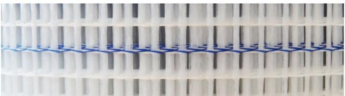
The basic fiber glass is obtained with the fiber technique (tecnica del fibraggio). Glass fibers are obtained by reacting mixtures of inorganic materials at temperatures above 1000 ° C using special furnaces. When the melted glass comes out the furnace it is processed in platinum chains through which it is stretched in the desired diameter so as to obtain a very small diameter filament. Yarn is obtained by the combination of a series of filaments.
